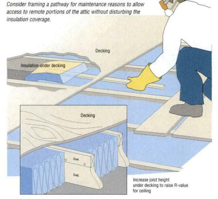
Installing insulation under existing attic decking requires some improvising to avoid removing the decking. Be sure to wear proper protective gear and clothing when installing any insulation. Install batt insulation with the vapor barrier down in attics with no insulation. If adding insulation on top of existing insulation, use batts without a vapor barrier backing or remove the backing.
