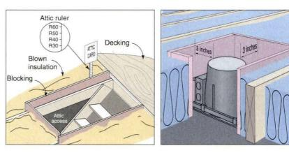
Attic rulers are required for loose-fill insulation and are a helpful guide to ensure adequate coverage. Create dams to hold back insulation and to maintain levels. Attic access such as scuttles and drop-down stairs benefit from a insulated cover.
