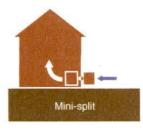
installed as wall-mounted ductless units (although short ducted runs are possible), and offer potential for zoning. They are ideal for conditioning additions and smaller zones such as bonus rooms. Ductless mini-splits usually heat and cool a room or two while ducted models can provide comfort to an entire home. Certain manufacturers offer variable speed and capacity units which can result
