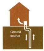
A ground-source heat pump (sometimes referred to as a geothermal heat pump) is a more efficient approach than air-source heat pumps. Instead of an outdoor condensing unit, ground-source heat pumps rely on buried pipes filled with water or other fluid to transfer heat between the ground and the house. Ground-source heat pumps are more
