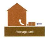
A packaged system has the air conditioner and furnace or the heat pump components contained in one larger outdoor metal box. There is one large supply and return duct connection from the outdoor equipment to the home's duct system.
